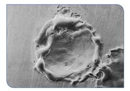
roll barrel surface area is fully covered with a consistent and repeatable texture, which has no directionality. It is this stochastic, isotropic surface which is so highly prized by automotive OEMs and other applications that require the highest quality textured sheet.
